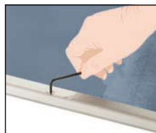
2. Allen key locking mechanism.
